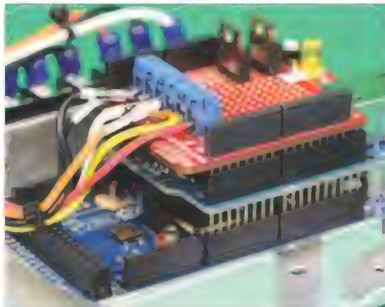
■ PHOTO 9. Arduino Mega 2650 with SparkFun protoboard.
